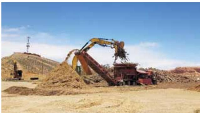
Grinder (Lance Excavating, Inc.) grinding green waste into unscreened quality mulch at Moab Landfill. Landfill located at 1282 Sand Flat Rd
