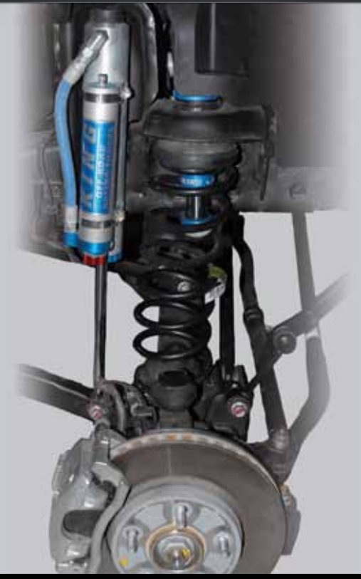
JEEP WRANGLER 2.5 W/WIDE RANGE COMPRESSION ADJUSTER SHOWN WITH JK BUMP STOP
